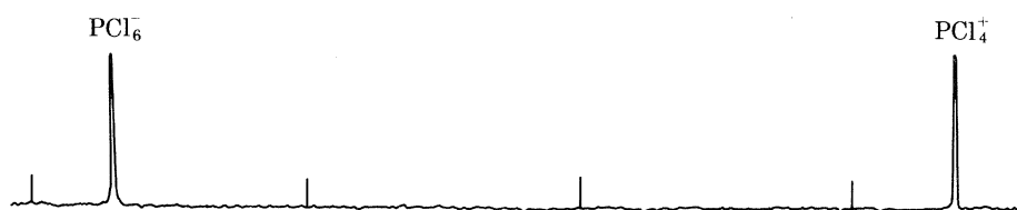
FIGURE 7. ^{31}\text{P} n.m.r. spectrum of polycrystalline phosphorus pentachloride with magic angle spinning. The two lines arise from the differently shielded \text{PCl}_4^+ and \text{PCl}_6^- ions of which the solid is composed. Markers at 1 kHz intervals (Andrew et al. 1960 a, b , 1966).
